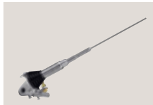
AH-2b ANTENNA ELEMENT A 2.5m long antenna element for mobile operation with the AH-4. All amateur bands between 7-54 MHz can be matched.
