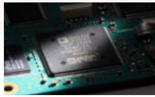
<DSP unit> ADSP-21369 Internal clock speed: 333MHz 32-bit floating point DSP Max. performance: 2000MFLOPS
